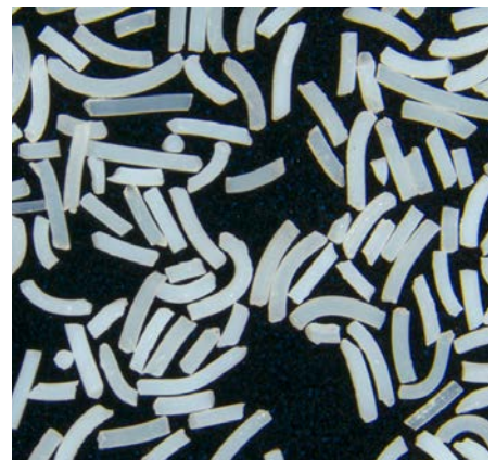
Rod-shaped ceramic grains for high stock removal
