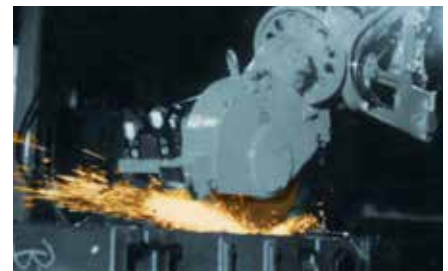
Machining of castings with grinding manipulators
